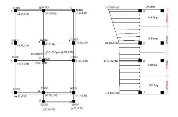
For strip A-A with 2.45m width and span 3.9m having soil pressure 118.76KN/m<sup>2</sup>
